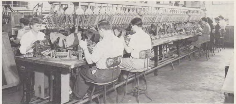
Employees adjust and assemble vertical connectors for Crossbar switches in March, 1954.
