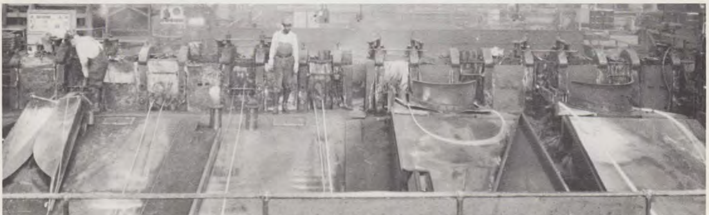
The looping mill, a spectacular operation in Hawthorne's Rod Mill of the 1960's, needed men with nerves of steel to work as catchers and guide the hot copper rods into drawing machines.
