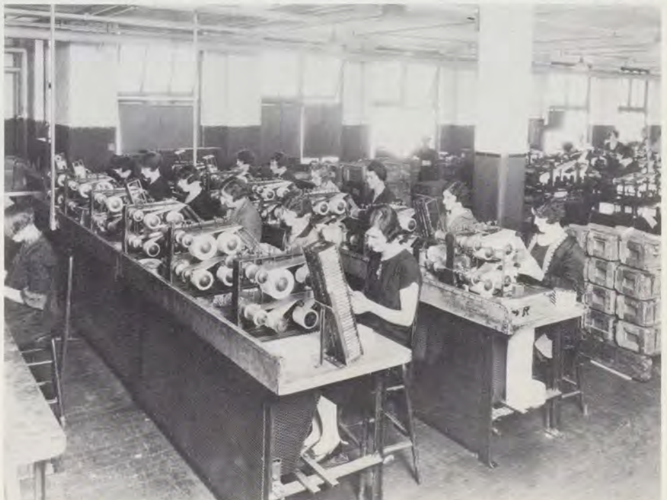
Hawthorne women employees here are operating condenser winding machines, one of the early jobs for women at the burgeoning factory. This photo appeared in the WE News in December, 1926.
