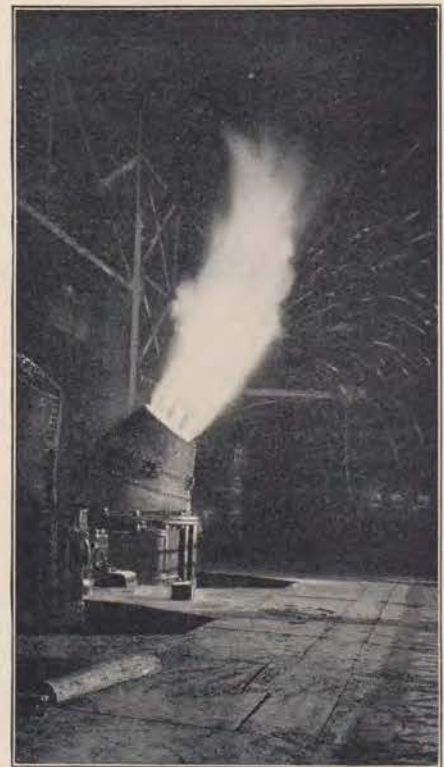
A modern Bessemer Converter in action. Hot metal from the blast furnace is poured into the pear-shaped converter and air is blown through for a short period, burning out the various impurities and converting the metal into Bessemer Steel.
