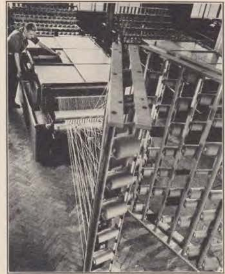
This machine glazes or coats the individual cotton threads with a starch compound which by producing a smooth, hard finish imparts to the yarn increased strength and resistance to wear. Glazed cotton is used in the outer covering of switchboard cords because this class of cord is subject to very severe usage in the telephone exchange.
