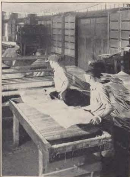
Straightening sheets of aluminum by rolling them.
