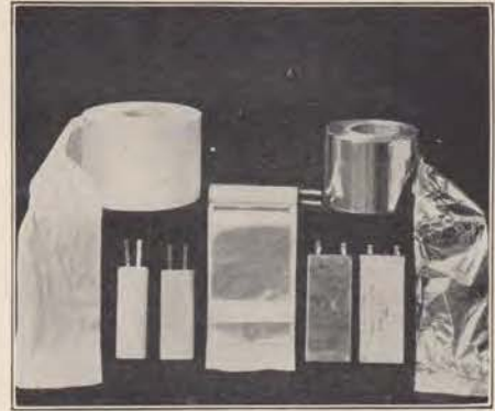
Aluminum foil is used in the manufacture of condensers. At the top are rolls of insulating paper and foil; in the center a condenser unit, slightly unrolled; while in the lower view are (left to right) a condenser unit before and after baking and waxing; a potted condenser before cleaning and painting—the unit having been inserted in a can which was then filled with asphalt compound; and at the extreme right the finished product.
