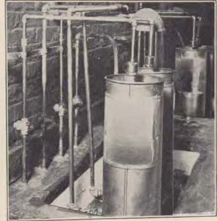
Carefully selected coal is used in the transmitter of your telephone. The operations of washing granular carbon are performed with the simple machinery shown above.
