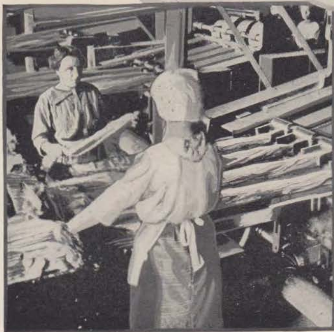
Spreading flax fibres on toothed belts to convert the separate fibres into continuous even sized yarns.
