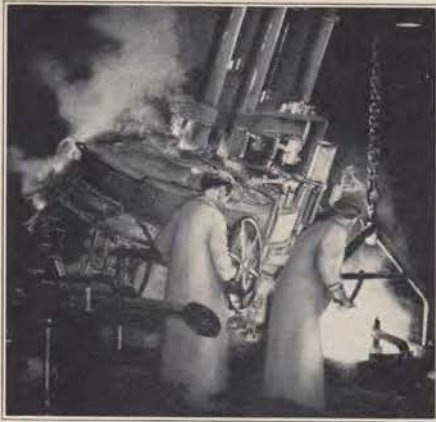
Molten nickel being discharged from a modern furnace into a special hopper.
