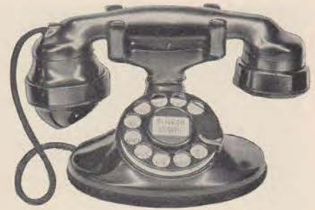
Copper is used in your telephone as an alloy in the brass for plates and screws and as bronze in the conductors of the connecting cords.
