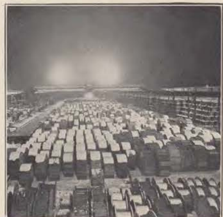
In the yard of the world's largest telephone factory an overhead traveling crane picks up heavy reels of lead covered cable and carries them the length of the yard or across it in a very few minutes.
