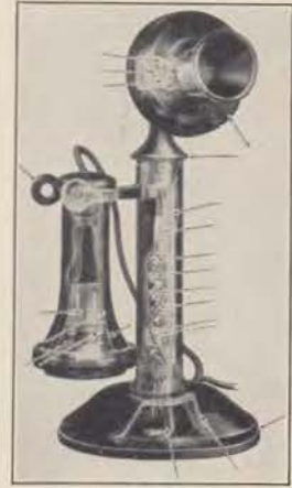
The brass in your telephone instrument contains zinc and zinc is also used to galvanize parts susceptible to moisture and other atmospheric conditions.
