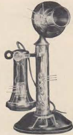
Nickel is sometimes used as a protective coating on the parts of the transmitter indicated by the three upper arrows and as plating on connectors in the receiver and for springs in the body of the instrument.
