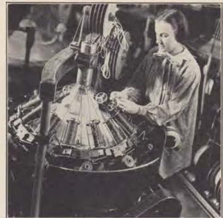
Cotton braid protects many types of telephone cords. As the insulated wires or cords come up through the center of this machine, spindles of cotton thread move round and round braiding on the protective layers.
