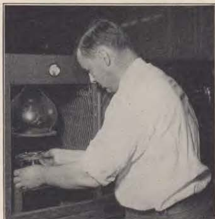
"Sputtering" gold on the diaphragms of broadcasting transmitters. The telephone handset transmitter electrode (terminal) and the interior of the tiny carbon cup are gold plated to provide a non-tarnishing surface, which is low in electrical contact resistance.
