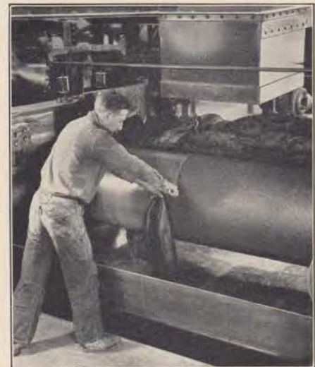
This heavy duty roller mill is used in processing various rubber insulating compounds for the manufacture of rubber covered wire. This operator is removing a batch of insulating compound preliminary to straining it through a fine screen to remove foreign particles.
