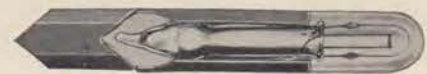
A side view of a switchboard lamp. In these lamps platinum-sheathed nickel-iron wires run through the glass. Platinum is used because heat and cold affect it to about the same degree as glass and therefore the wires do not shrink away from the glass and let air into the lamps.
