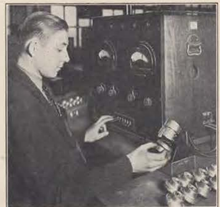
Each handset transmitter is placed in a volume testing machine, equipped with an oscillator that delivers through a telephone receiver all the sound frequencies that are essential to perfect speech transmission. The machine, in turn, indicates by means of a vacuum tube circuit the degree to which the transmitter responds to the various sound frequencies.
