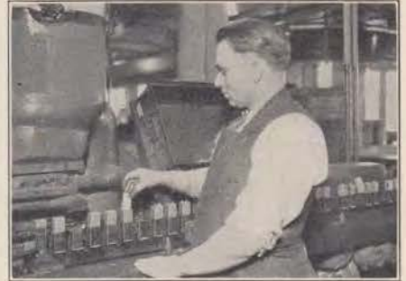
A condenser "potting" operation in which the condenser cans are filled with asphalt compound, and the units, composed of wound alternate layers of aluminum foil and paper, are inserted.
