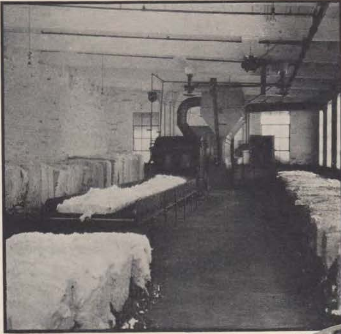
Left—A cotton breaker which opens the bales at the mill.
