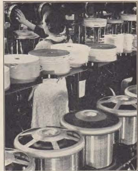
A row of paper insulating machines. The shiny copper wire shown on the spools in front of these insulators is wrapped with insulating paper much like one would tape a baseball bat, except that very close limits must be maintained.
