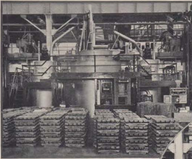
Right—Antimony charging mechanism of a centrally controlled lead melting system.
