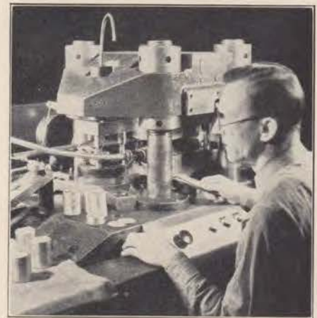
Diaphragms for telephone transmitters are blanked, formed and perforated out of strips of the aluminum alloy by machines like this.
