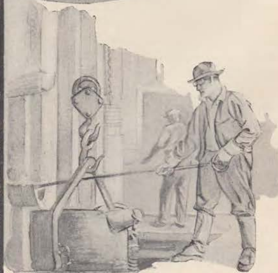
Open-hearth furnaces used in making aluminum alloys. Furnace in the foreground is being tapped.
