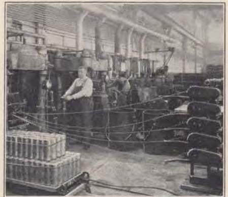
In these presses, thin, hollow, lead-tin piping is filled with rosin to make easy-to-use rosin core solder.
