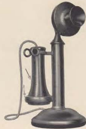
Sheet rubber baked and vulcanized is used for the receiver of the desk stand telephone and molded rubber dust is used to form the cap of the receiver.
