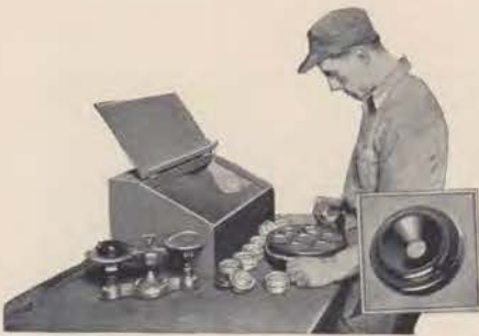
Rubber dust is poured into molds like the one the operator has before him and dies are inserted in powerful presses. When heat and pressure have vulcanized the rubber contents of the mold, receiver caps result, ready to be smoothed to the glass-like surface you have so often felt against your ear.
