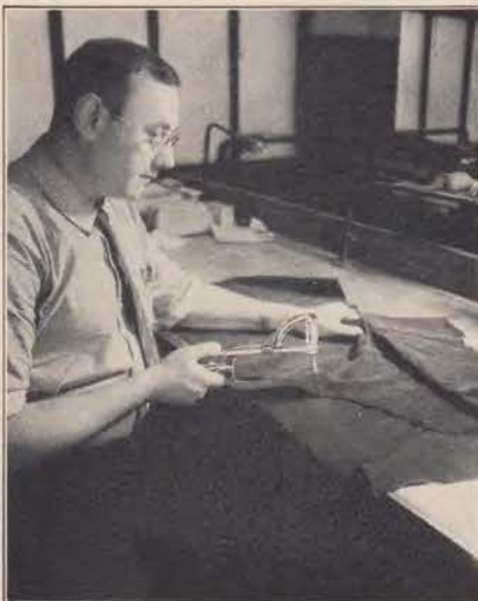
Determining thickness of sanded leather used for base of telephone handsets.
