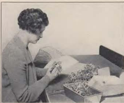
Inspecting telephone parts. Nickel is used as a finish on many of the parts used in telephone apparatus to insure resistance to atmospheric effects.
