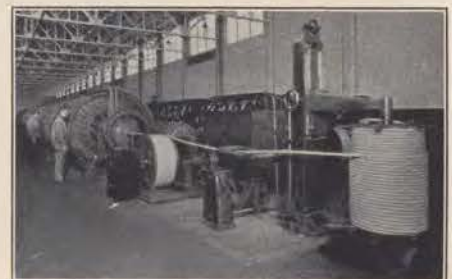
Cable making. A cable 2½ inches in diameter contains as many as 1,818 pairs of copper wires.
