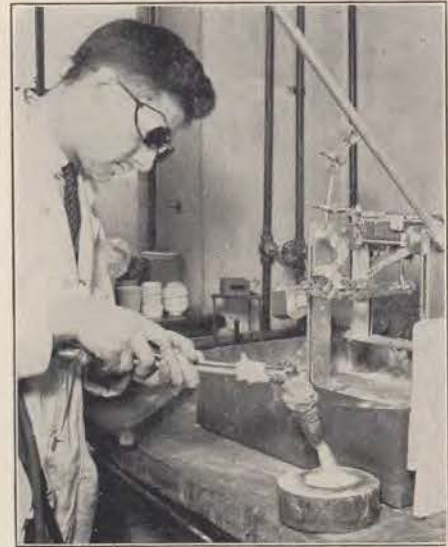
Pre-melting platinum sponge. "Sponge" is really a misnomer because at this stage of the recovery process, it is a powder which must be melted prior to casting into ingots.
