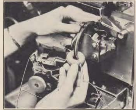
Winding enameled wire, further insulated with cotton, around magnetic cores—used in loading coils which play an important part in long distance telephony. Cotton used in insulating wires, is first purified by special washing processes to remove any soluble salts.
