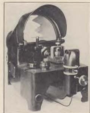
Apparatus for checking the accuracy of threads on phenol plastic receiver caps. An enlarged image of the threads is projected to make certain they are within limits. This care is necessary because telephone parts must be interchangeable.
