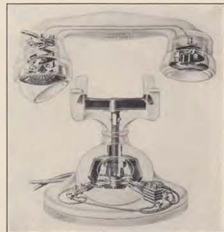
The cord emerging from the handle of this telephone set, those seen inside and those connecting cords (see text) coming from the base of the stand are covered with an insulation made of cotton.
