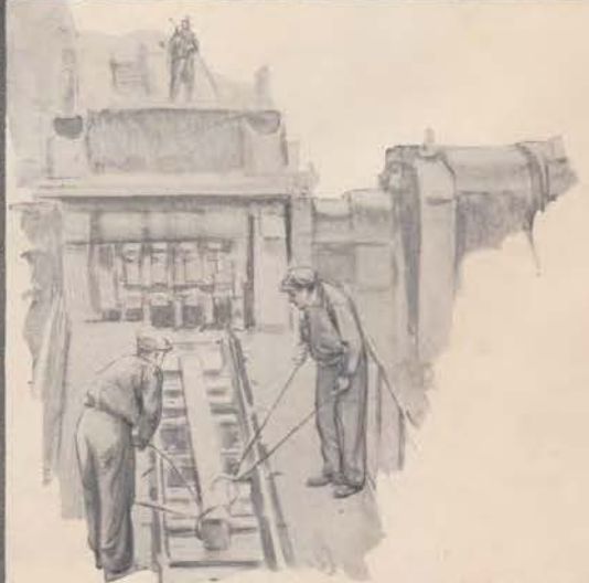
The blooming mill handles the steel ingots as the blacksmith with his hammer and anvil shapes small pieces of iron and steel.
