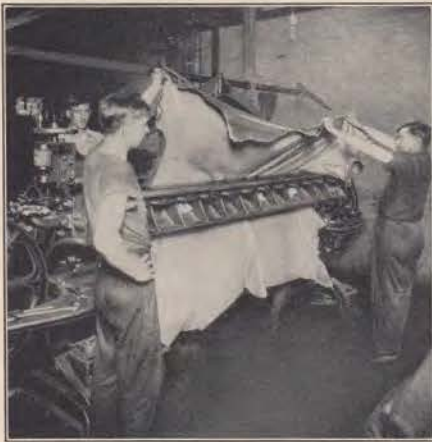
Splitting the hide. This delicate and interesting operation separates the grain which carries the hair from the hide and also splits the hide into various thicknesses.
