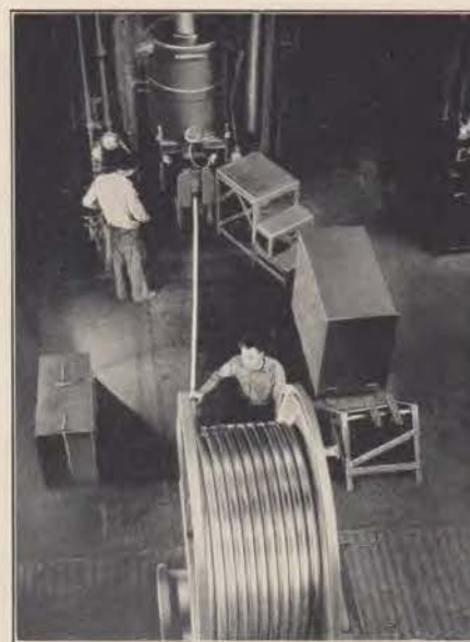
Covering a cable with lead and antimony alloy sheath at the Point Breeze works of the Western Electric Company.
