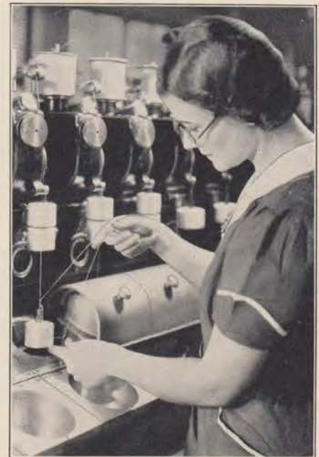
Silk is wrapped around fine copper wire in a serving machine pictured above. The operator is adjusting the silk band to assure perfect coverage of the wire.
