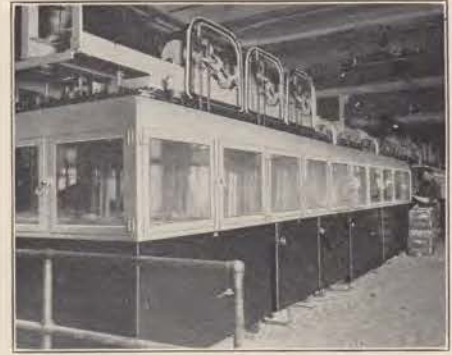
Zinc plating, a process that protects iron from moisture and rust, is done by immersing the parts to be coated in a plating solution and depositing zinc on them by electrolysis.
