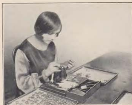
A round piece of mica forms one end of the carbon transmitter button of your desk stand type telephone instrument.
