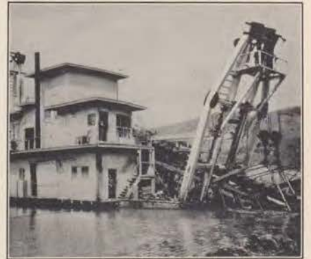
Dredges are now the chief means by which alluvial gold is recovered. Here is a large unit at work in Oregon.
