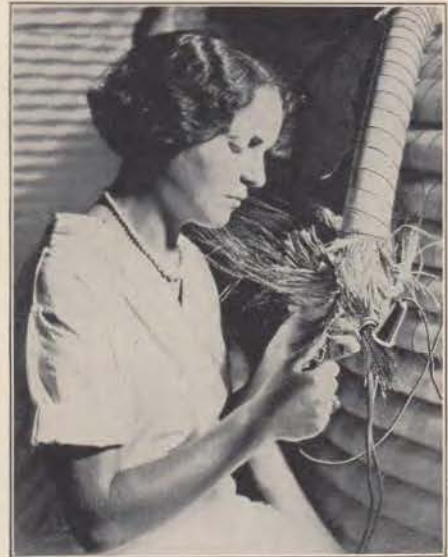
This shows the paper wrapped wires in a cable and the paper wrapping around the entire rope-like group of wires, just as the cable core looks before it receives its sheath of lead and becomes real lead covered cable.
