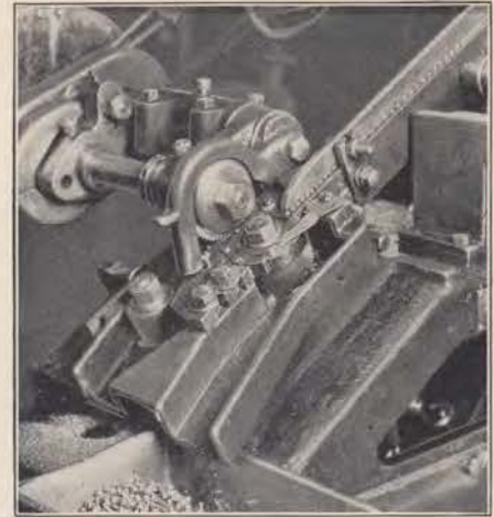
This automatic machine is one of a series of three which make iron screws; the first draws in the iron rod, forms the head and cuts off the proper length; the second slots the head; the third forms the thread. This is the machine which cuts the slots in the heads.
