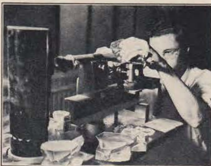
With this polariscope the trained worker determines exactly the axis of the quartz crystals before they are diamond sawed and then ground within extremely small tolerances.
