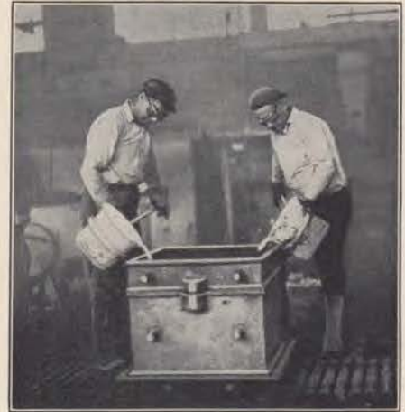
Pouring magnesium sand castings. Because of the great consumption of electric energy, magnesium, like aluminum, is produced where power is cheap.
