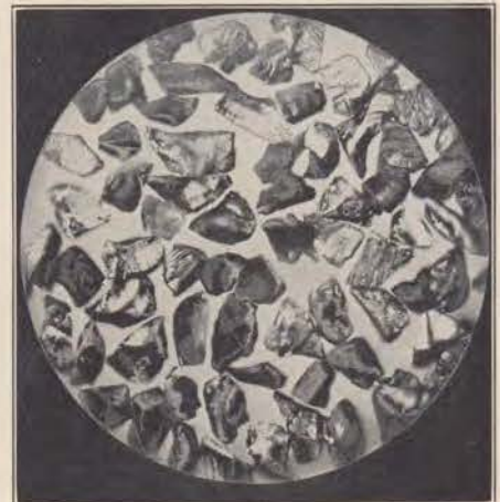
Granular carbon, greatly magnified, as used in telephone transmitters.
